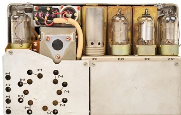
PR-56A rear view showing RF unit left and other stages right.
